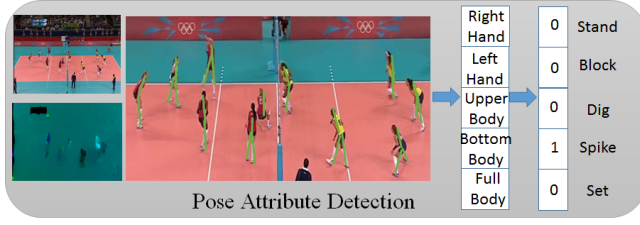
Figure 3: Pose attribute detection part in our model. The inputs are both RGB and optical flow images, and the outputs are binary representation of semantic attributes.
